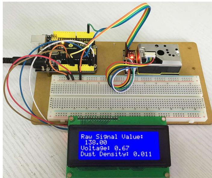
Result of Project 2: Open serial monitor, displaying as following.
